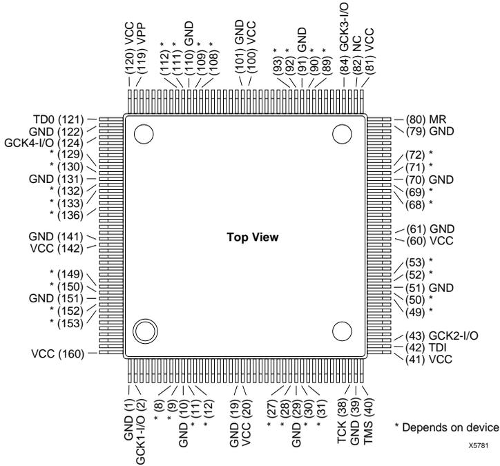
Figure 26: PQ160 PQFP with 160 Leads, .65mm Lead Pitch
