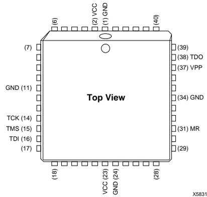
**Figure 22: PC44 PLCC with 44 Leads, 50 mil Lead Pitch**
