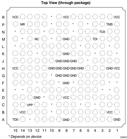
Figure 27: BG225 Plastic Ball Grid Array with 225 P<sub>b</sub>S<sub>n</sub> Balls, 15 x 15 Array, 1.50 mm Lead Pitch
