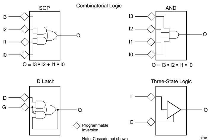
**Figure 5: Programmable Cell**
