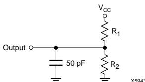
4. Output delays (except input E to pad O begin hi Z) change with capacitive load according to the following table. Delays above are calculated for 50 pF. As an example, `obuf_ir` at 20 pF is:  $3.4 - (30 \times 0.21) = 2.77$  ns. XC8100 software can make these calculations automatically.
