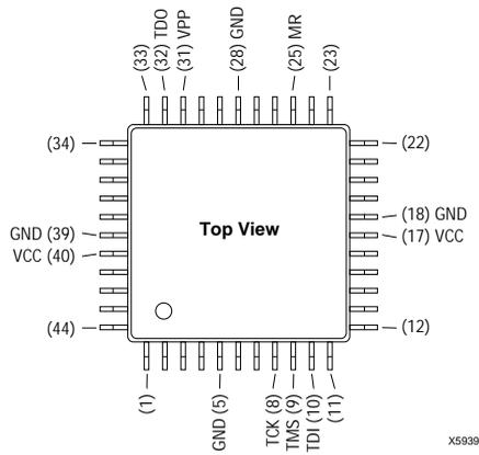
**Figure 23: VQ44 VQFP with 44 Leads, 0.8 mm Lead Pitch**
