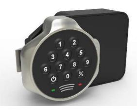
**Smart security locks.** The lock was designed (hardware and software) to be accessible via electronic keypad, unique RFID card, NFC on a mobile phone, fob, or wristband;
