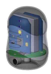
**An IoMT stethoscope device** for heart, respiratory systems and blood vessel diagnostics.
